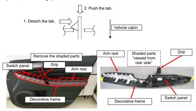
6. For door trims fitted with a grip, remove the grip from the decorative frame by detaching the 2 tabs.
