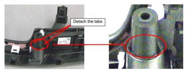
7. Remove the switch panel from the decorative frame by detaching the tabs.
