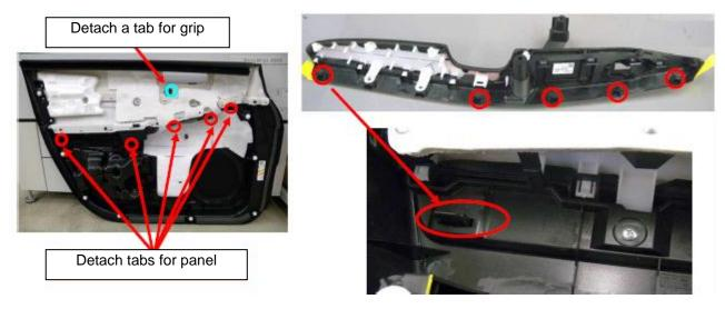
5. Detach & push the tabs (see below), then pull the frame starting from the rear of the frame and moving to the front, remove the frame from the door trim. The frame, switch panel, arm rest and grip will be removed as one unit.
