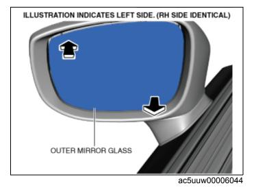
5. Insert your fingers into the area shown in the figure, and move the outer mirror glass in the direction of the arrow to detach pin A.
