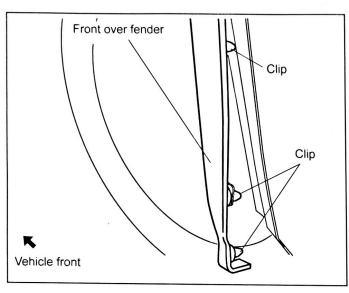
5. Remove the front over fender clips in the three locations from the bottom.
