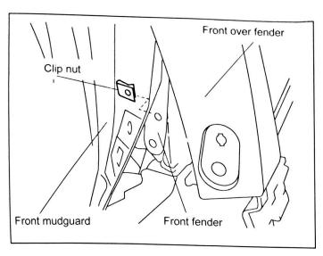
Peel back the front mudguard and front over fender, and install the clip nut to the position shown in the figure of the front fender.
