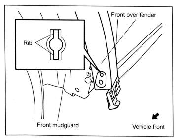
6. Cut out the rib of the front over fender shown in the figure using a nipper.
