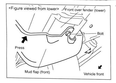
12. While pressing the mud flap (front) in the direction of the arrow in the figure, securely tighten the bolt so that there is no gap between the contacting surface of the front over fender (lower).
