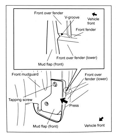
11. Press the mud flap (front) in the direction of the arrow in the figure so that the gap between the contacting surfaces at the upper/lower area of the V-groove are uniform. Securely tighten the tapping screw so that there is no gap in the contacting surfaces with the front over fender and front over fender (lower).
