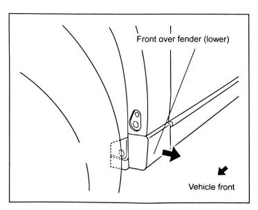
Grasp the flange on the vehicle interior side of the front over fender (lower) with your hand, pull it in the direction of the arrow and remove it. (Front over fender (lower) is secured by tabs in three locations.)
