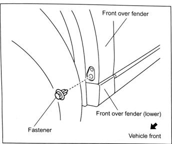
Re-install the front over fender and front over fender (lower) to their original positions and only install the one reusable fastener removed in Step 1.
