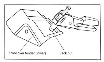
4. Install the jack nut to the hole on the underside of the removed front over fender (lower).
